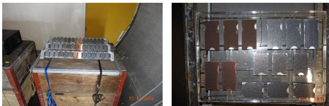
Figure 15 Corrosion monitoring in tunnel ‘A’
